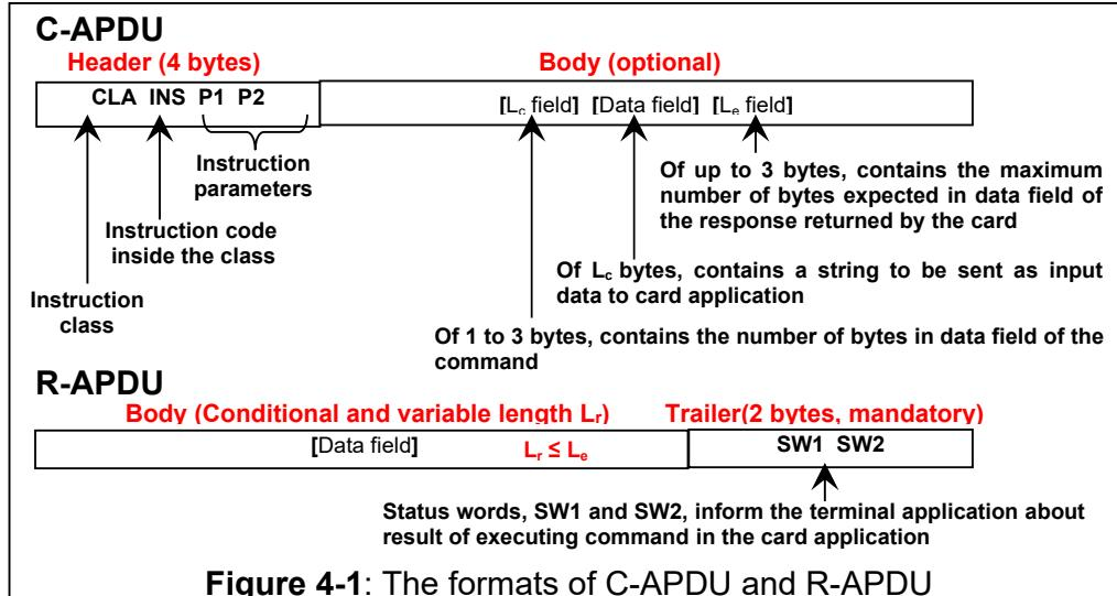
**Figure 4-1:** The formats of C-APDU and R-APDU
